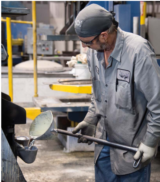
A Batesville Products employee pours molten aluminum into a mold at the company's foundry near Lawrenceburg, IN.
